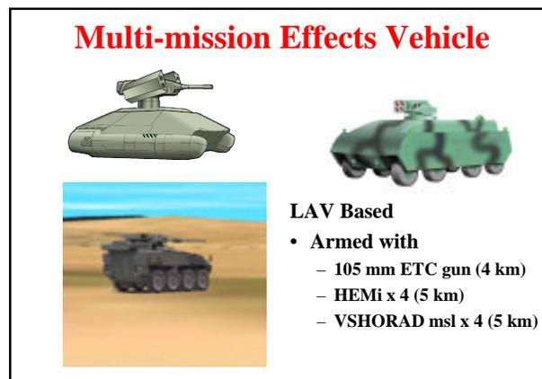
vehicle was modelled on the capabilities inherent in the FAV project. Armament consisted of a 105 mm electro-thermal-chemical gun with a basic load of 40 rounds and a pod mounted missile system for both anti-tank and VSHORAD tasks.
