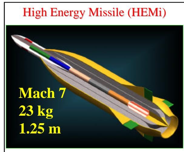
approximately one meter in length, weigh 20 kg and reach a speed of mach 7 within 400 m of launch. Given the speed of the missile, it is expected that it will be a laser beam rider.
